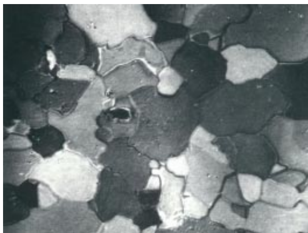
Fig.b: Structure of steel
