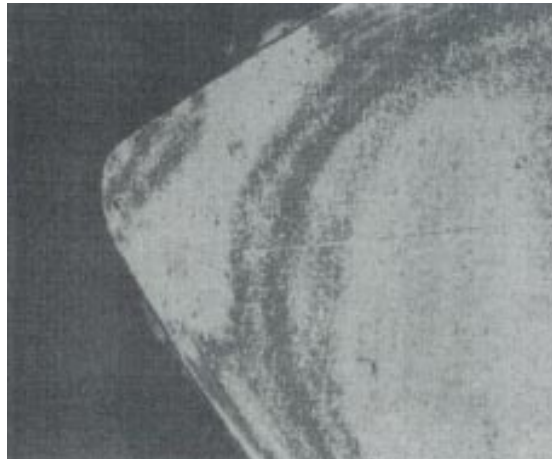
Fig. a: Apart from a void ( air inclusion), the tip of a gear wheel also exhibits material inhomogeneities (consolidations),
